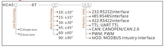
E.g: HCA516T-10-232: Single axis/Standard /±10° Measuring range/ Data interface port RS232
